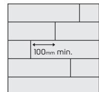
Tile products should be laid in a brick bond to give the floor maximum stability and enhance the aesthetics of the floor.
