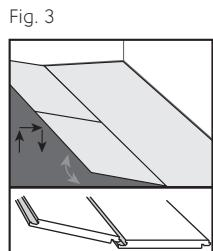
Step 5. Fit the next tile or plank by clicking the tongue and groove together along the short edge. Ease the tongue and groove together on the long side by angling the tiles/planks together.
