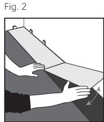
Step 4. Start the second row by clicking the tongue into the groove holding the tile or plank at an angle (approximately 30°), then push the tile or plank firmly into the groove of the first row. (Fig. 3)
