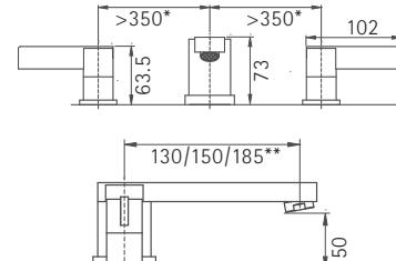
\* Flexible hose enables variable mounting distance - up to 350mm.
